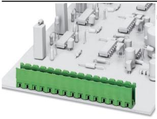
Header, nominal current: 12 A, rated voltage: 250 V, pitch: 5.0 mm, no. of positions: 9, mounting: Soldering
